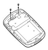
6 Pull the cord connecting the battery to the player to separate the battery plug from the connector.
